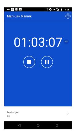
15. The user is forwarded to the Time info view and the device location is determined to end the work time. If desired, the user can change the objects or add a comment. The work time is ended by pressing the "End" button at the top right corner of the screen. The user is then forwarded to the timer home screen, where a new work time can be started.
